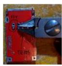
sit flatter down on the PC-6. No tape or insulation needed on U1.
