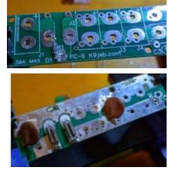
9. Assemble U1 power input using the legs trimmed from D1 above. Tack-solder these in place as shown. Except for the +5V output pin, trim off the USB connector pins on U1 that stick through the board so they are flush to the bottom of the board. This is so it will sit flatter down on the PC-6. No tape or insula
