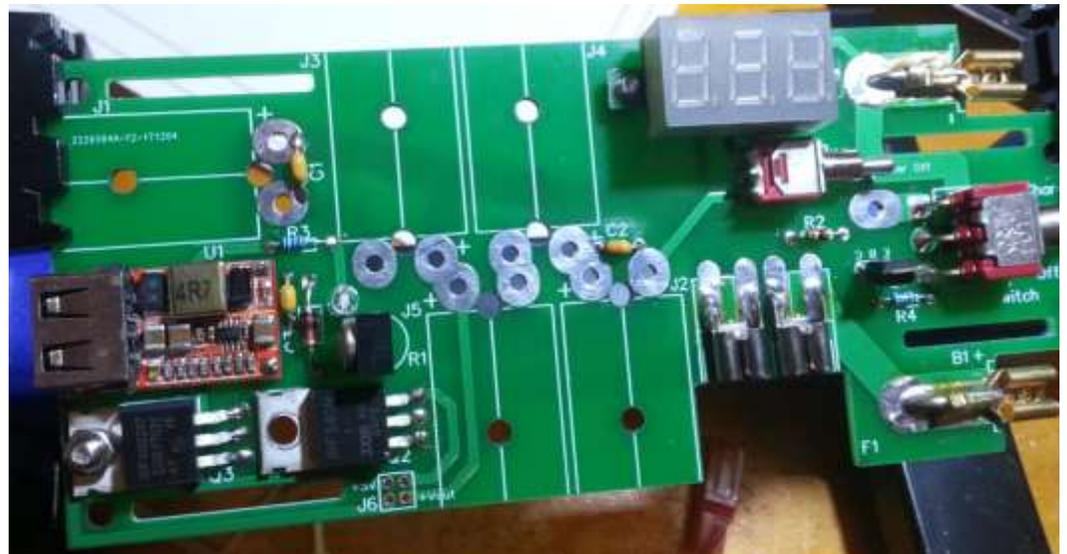
from the back side of the board so the solder flows through the holes and fuses with the meter contacts. Test the meter by switching the switch to Vin and applying voltage to J5, confirming the meter works.
